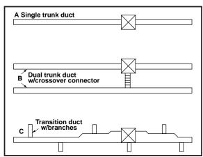
Figure 2. Non-Platinum Supply Duct System
